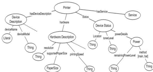
Figure 2: Printer Class Example
