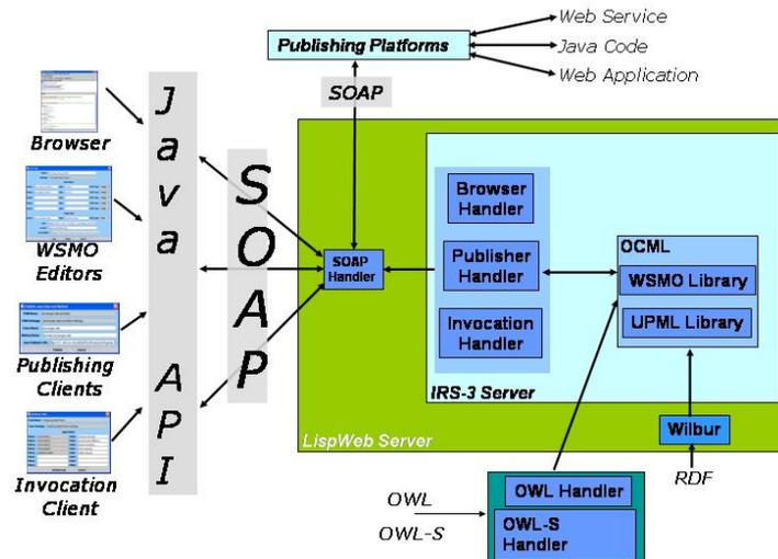
Fig. 1. The IRS-III Server Architecture
